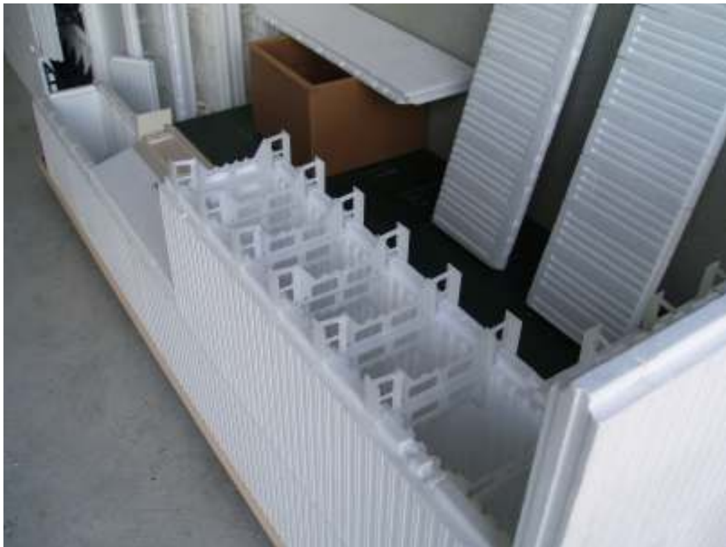
INSULFORM Supa Block – Fully Patented heavy duty polypropylene bridges set at 125mm centres (8 per block)
